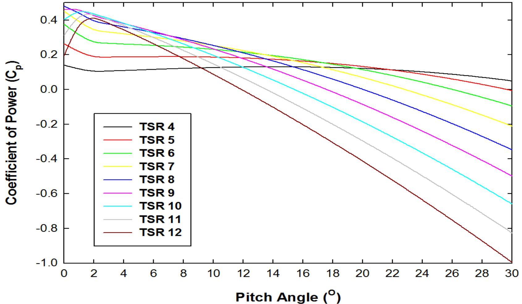
[Coefficients of Power vs. Pitch angle according to TSR(Tip Speed Ratio)]
