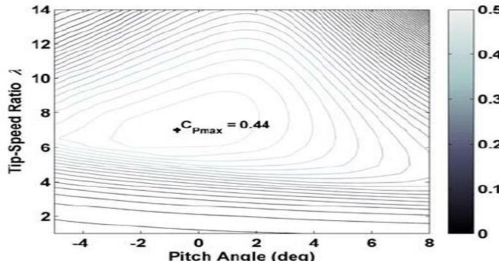
Variation of the power coefficient  $C_p$  as a function of the blade pitch angle  $\beta$  and tip speed ratio
